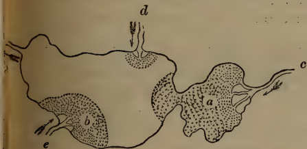
FIG. 123.—PLAN OF A LAKE ENTERED BY THREE STREAMS (c, d, e), EACH OF WHICH DEPOSITS A CONE OF SEDIMENT (a, b) AT ITS MOUTH.
